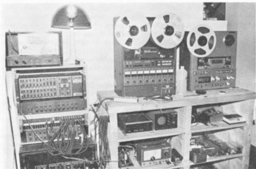
PHOTO #3 - Shown here is an Echoplex, Tapco and Techniques equalizers, Teac mixer, Eventide Instant Flanger, Teac 80 - 8, Sony TC - 880 two track, DBX noise reduction and miscellaneous test gear. A Yamaha 12 input mixer is also used.
