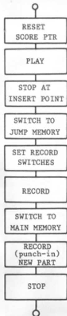
DIAGRAM #4 - Procedure used to overdub (punch-in) a new part.
