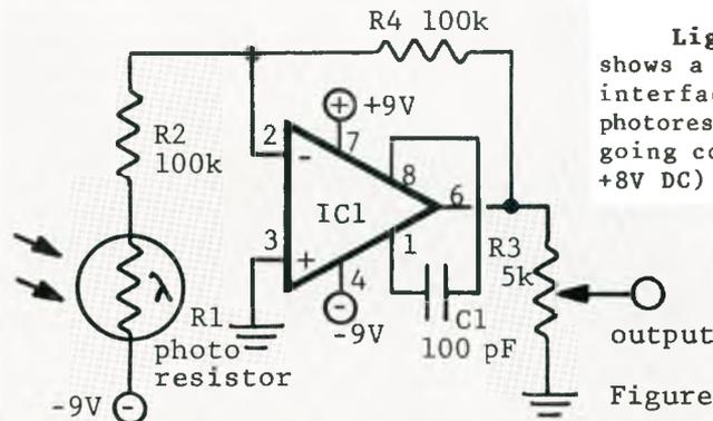
**Light Interface.** Figure 2A shows a simple but effective light interface. Light striking the photoresistor produces a positive-going control voltage (about 0 - +8V DC) at the output, which can
