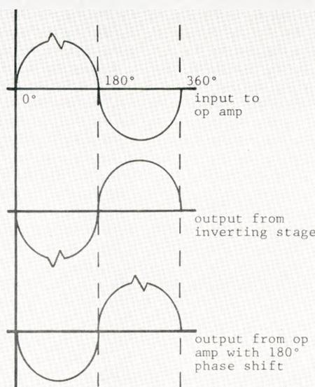
Figure 2: Inversion vs. Phase Shift
