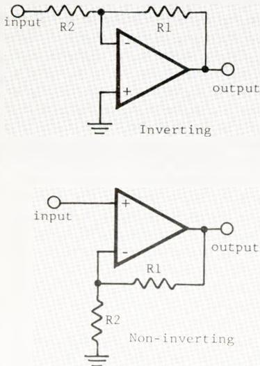
Figure 1: Op Amp Gain Stages
