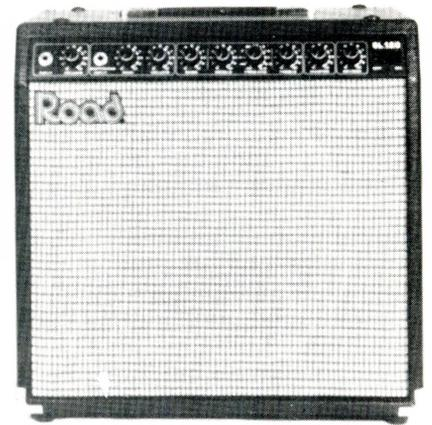
**Two New Guitar Amps.** Road Electronics (2107 E. 7th St., Los Angeles, CA 90021) has announced the SL120 lead amp with switchable channels and the L120, a single channel version. Both models feature 3 band active EQ, FX loop, master volume control, headphone jack, and 60 Watt RMS power rating.
