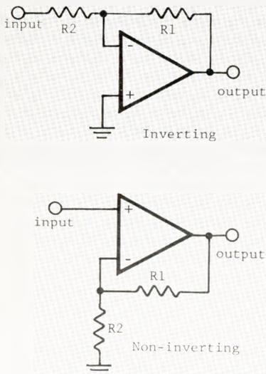
Figure 1: Op Amp Gain Stages
