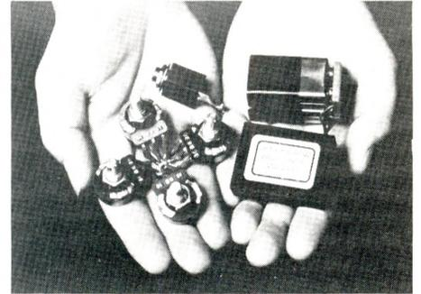
**For the Active Guitar.** A/DA (2316 Fourth St., Berkeley, CA 94710) now distributes the Little FEANC from Zeta Systems. Designed for on-board mounting in most electric guitars, the FEANC includes a Fuzz, Equalizer, Amplifier, Noise gate, and Compressor in a 1.5" x 2" by 0.5" package.
