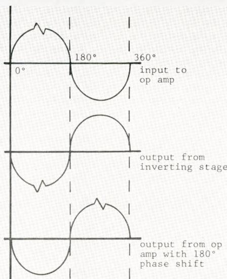
Figure 2: Inversion vs. Phase Shift
