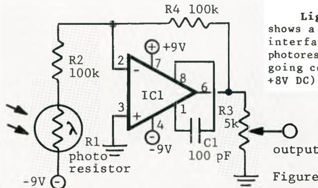
**Light Interface.** Figure 2A shows a simple but effective light interface. Light striking the photoresistor produces a positive-going control voltage (about 0 - +8V DC) at the output, which can
